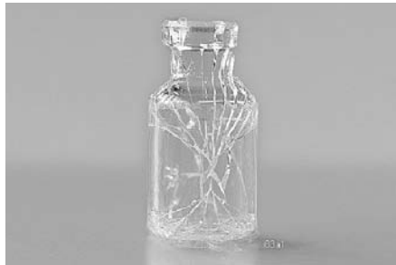
Broken vial after burst pressure test
