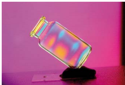
Stress distribution in vial that was not completely relieved after hot forming
