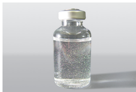
Corrosion effects: glass flakes
